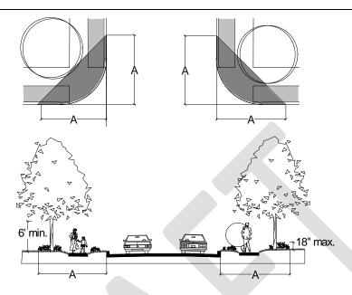
Note: A = Distance measured from street curb as set forth in Section 110.412.30 (c)(1), (c)(2), and (c)(3).
